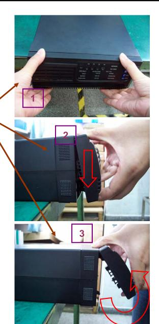
Remove the front panel for the top of plastic housing.
