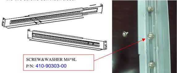
2). Fix the right nut (412-90029-00 or 412-90055-00) in the rack, and then align the slide-rail on both sides of rack by the screw holes, and lock a screw(410-90900-00) in the downside hole of both sides at the front of the rack.
