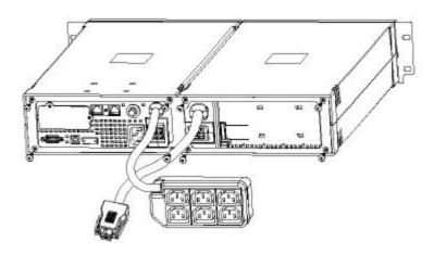
8) Setup rack-mount is completed and to connect the UPS
