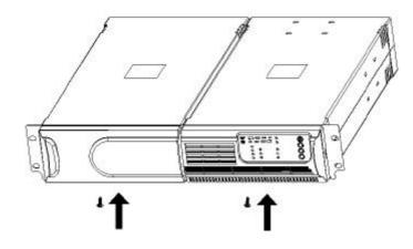
6) Setup rack-mount for front side is completed
