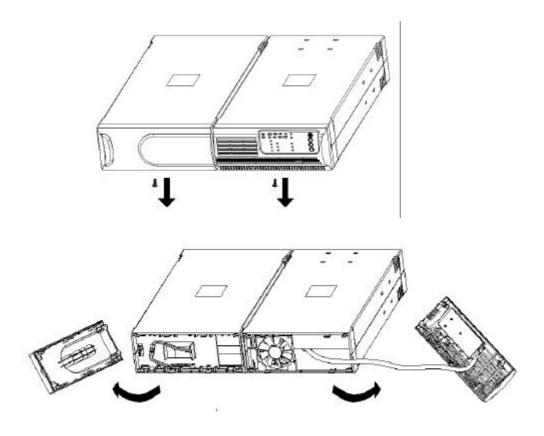
4) Align the mounting bracket with the screw holes on the each side of Host and EBM and secure with the supplied screws(410-90100-00).
