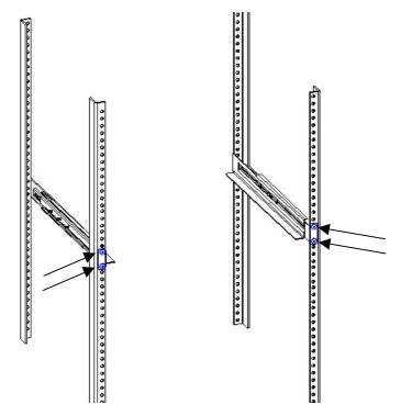
4. Insert UPS into the slide-rail and lock it(screws:410-90900-00) in the rack enclosure.
