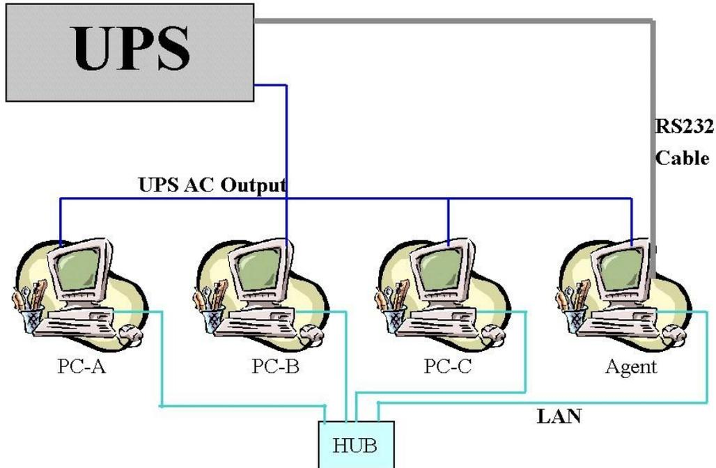
1. To support the remote monitor/control function of WinPower, you need to have the similar connection as above. It means that the Agent is connected to the UPS via RS232/USB and the other Computers are protected via the AC Power only; and all the computers are communicated under the same Network with LAN.
