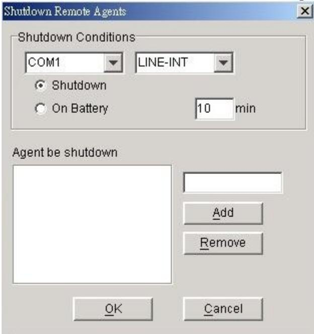
“Shutdown” means that when the UPS of the Agent is going to shutdown, WinPower will send out the shutdown command to the remote PC of the IP that you added in the space below.
